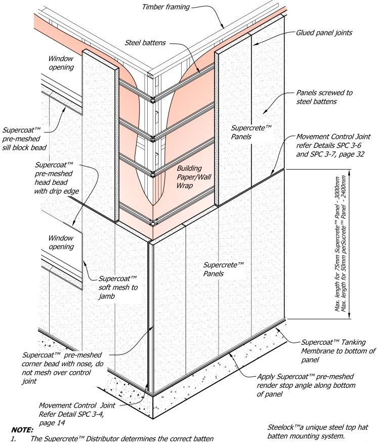
1. The Supercrete™ Distributor determines the correct batten spacing using wind and earthquake load information supplied by the building owner on the design documents
